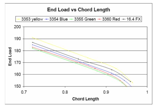
This was done with all carbon poles with a 16.4 flex. Doing this with a Skypole, Spirit, current Essx Carbon, Gill Composite and if you could find the same Weave 4B and 2002 version of the white Carbon FX would be an interesting comparison –
