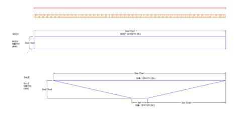
• Bottom pattern is from late 1970's Pacer - below is a snippet from the 2011 Pole Paper. This concept leads to longer short side of the sail – top of the trapezoid shown on above diagram of four different sail pieces. This concept is currently used by Spirit:
