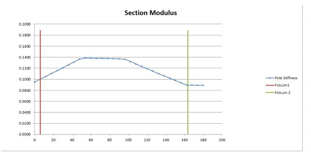
This illustrates how the sale portion effects the distribution of material. Since this is only a part of the pole and less than 50% when you consider initial layers (roving, spiral wrap, or veil piece) and the body wraps of the pole.
